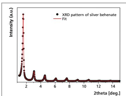
Another measure of performance is the linearity of the goniometer. A highly linear goniometer provides accurate peak positions over the entire 2theta range of the goniometer. This is important if you are making critical calculations from your XRD data, such as unit cell size of cracking catalyst. Linearity is determined using a line position standard such as [NIST 640e](#) – silicon powder. For the good peak position accuracy 2theta linearity should be within  $\pm 0.02$  degrees 2theta.
