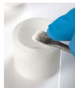
requires the addition of some binder. The resulting pellets can be analyzed without supporting film, and can also be analyzed in vacuum. The amount of binder added rarely exceeds 10% of sample mass, so the effect of the dilution is minimal.
