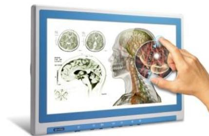
lying out on the glass sheet. Voltage is applied to this grid creating an [electrostatic](#) field. When the finger comes into contact with the screen it distorts the field at that point, measured as a change in [capacitance](#). This change in charge can be measured extremely accurately and even a gloved finger can be sensed by PCT. The sandwiched sensor grid allows even two to ten finger touch points for pre-defined gestures like pinching,
