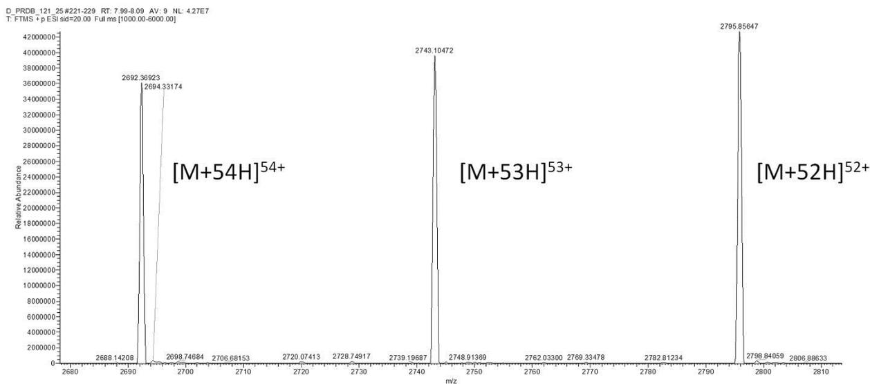
Figure 5: Mass spectrum of the deglycosylated antibody
