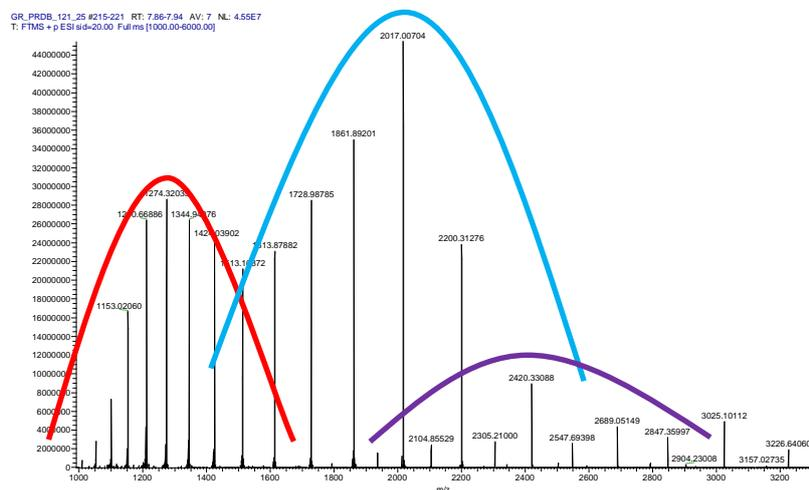
Figure 7: Zoom-in of the mass spectrum of the light chain indicating the three charge envelopes
