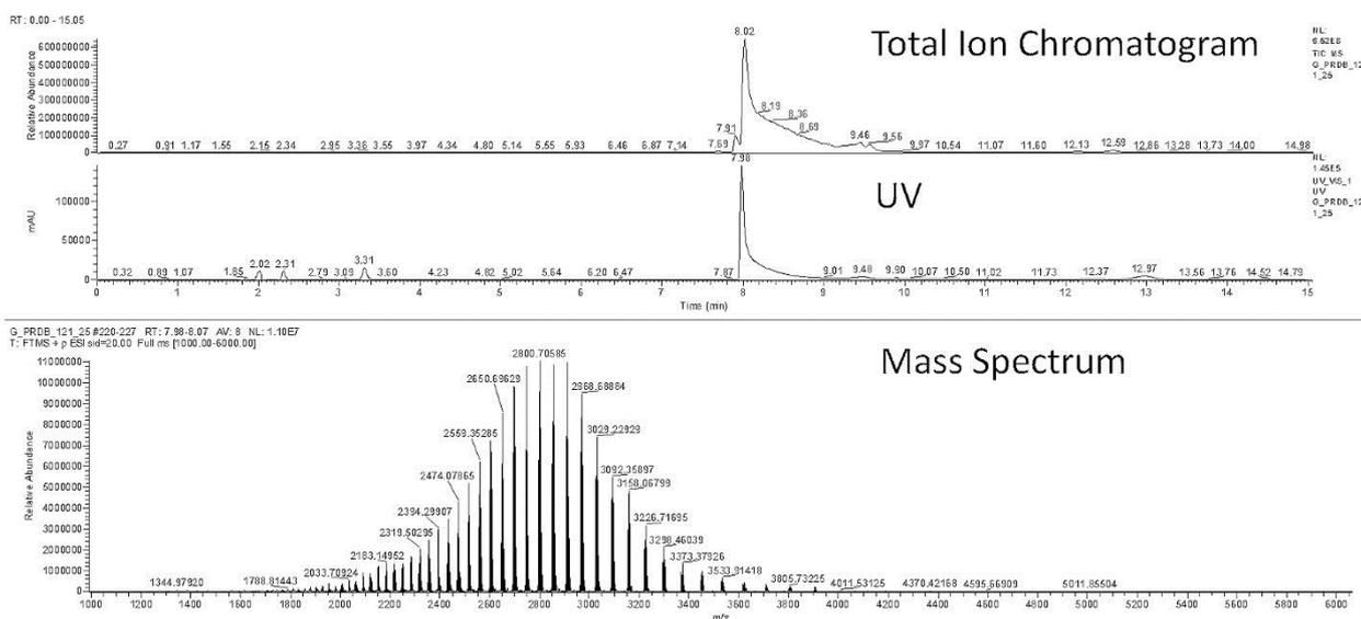
Figure 2: Mass spectrum of the intact, unmodified antibody
