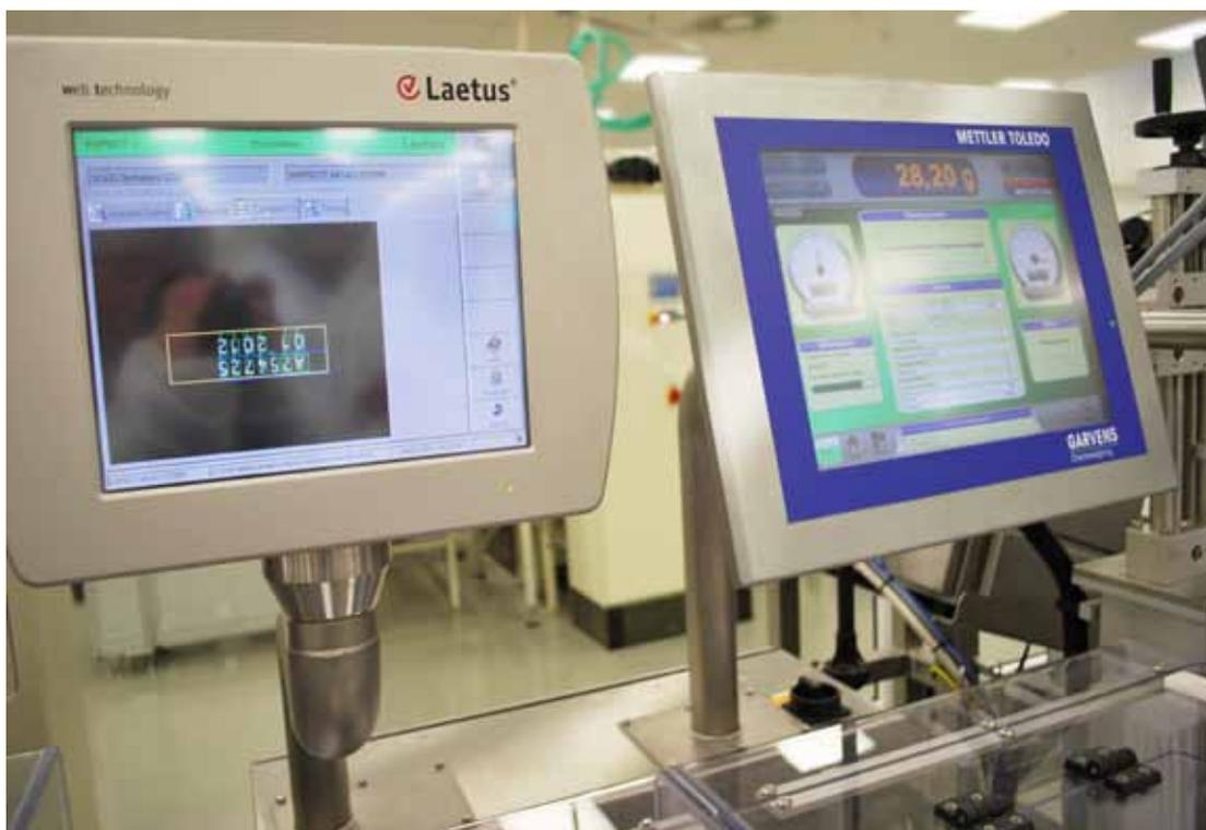
Print verification camera and laser marker operating terminal alongside the METTLER TOLEDO Garvens weighing terminal
