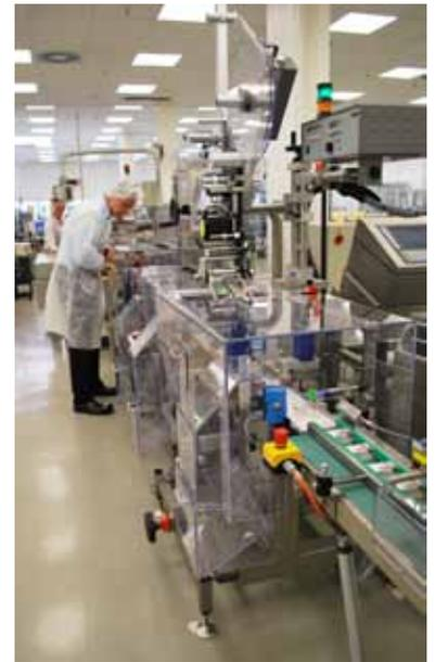
In the marking and verification process, secondary packaging is marked with a unique code to facilitate comprehensive forwards and backwards traceability of products from the packaging line right up to delivery to chemists or healthcare facilities.
