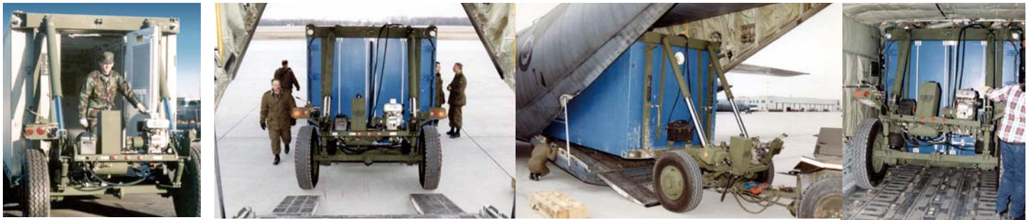
Rear Dolly Permits Full Opening of 3-4 ft Wide Access Doors. Dolly Set Loaded into C130 Aircraft with 8-ft. x 20ft ISO Container.
