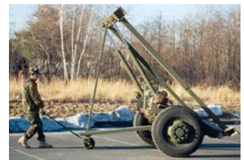
Dolly Set being Maneuvered in 3-Wheel Handling mode
