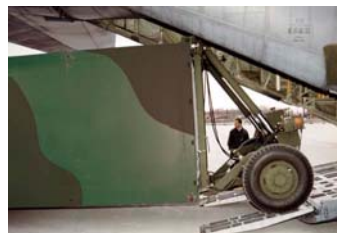
M1022-A1 Dolly Set Loading Shelter onto C130 Aircraft
